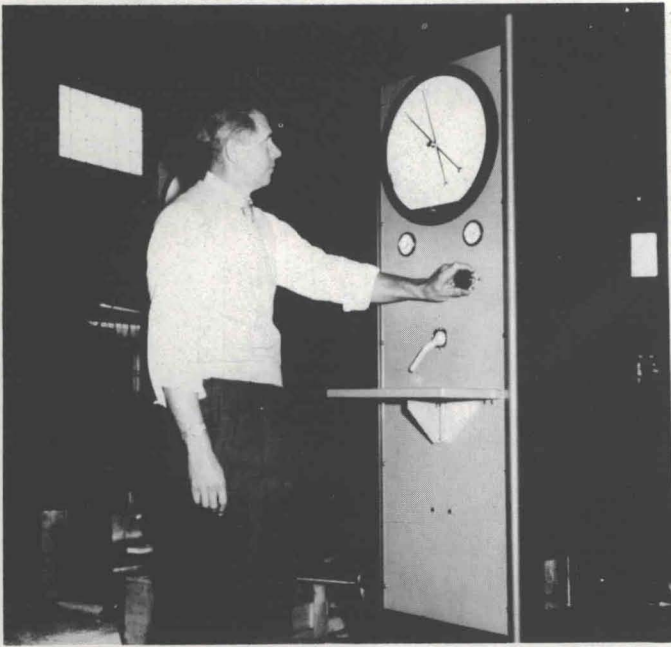
Fig. 20 Hinge unit control panel
