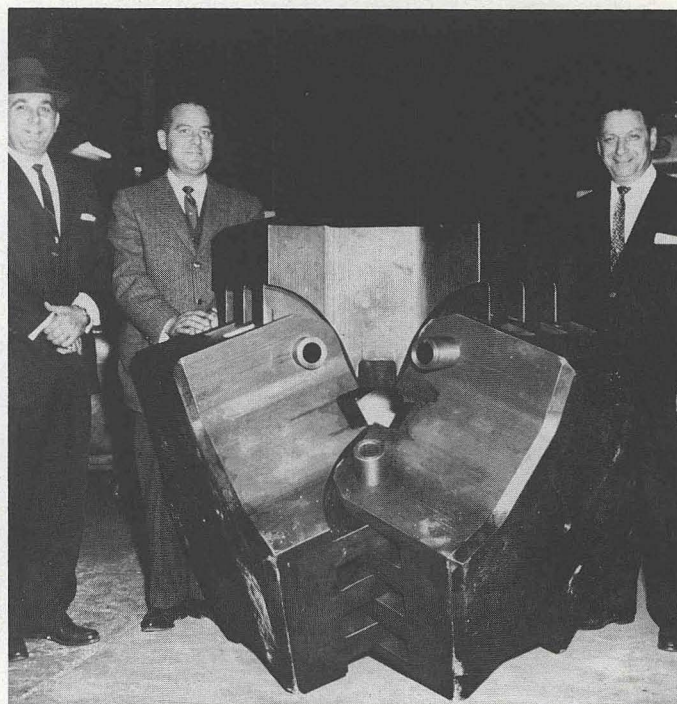
Fig. 19 Assembly of a 2000/8000 ton tetrahedral hinge unit
